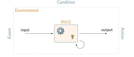
State-based ECA rules: "on movement if alarm = "active" then siren  $\leftarrow$  on" variables can be internal, or connected to sensors or to actuators
